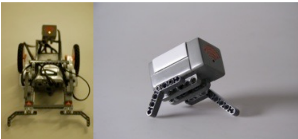
Figure 12: Pictures of the WifiBlock connected to ordinary lego pieces.
