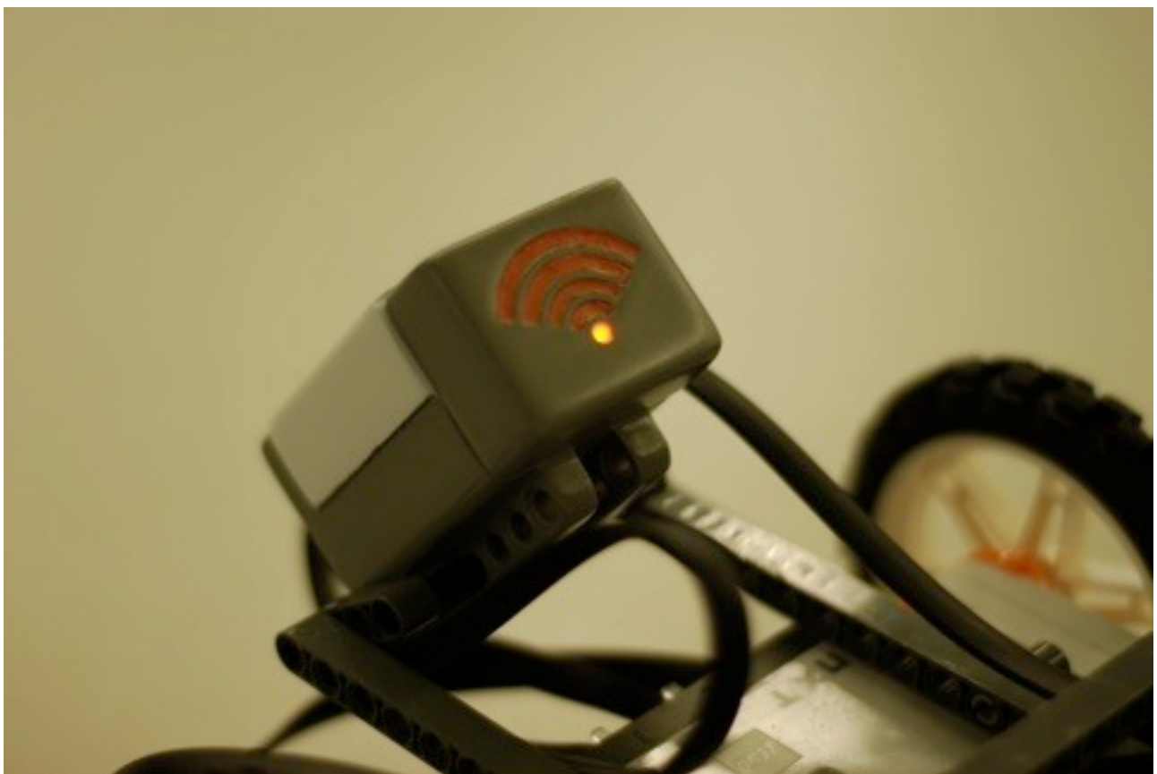
Figure 14: Led that indicates the WifiBlock has a connection to the internet
