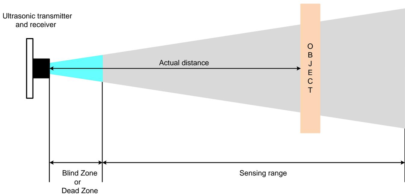
**Figure 18. Minimum and Maximum Measurable Distances**
