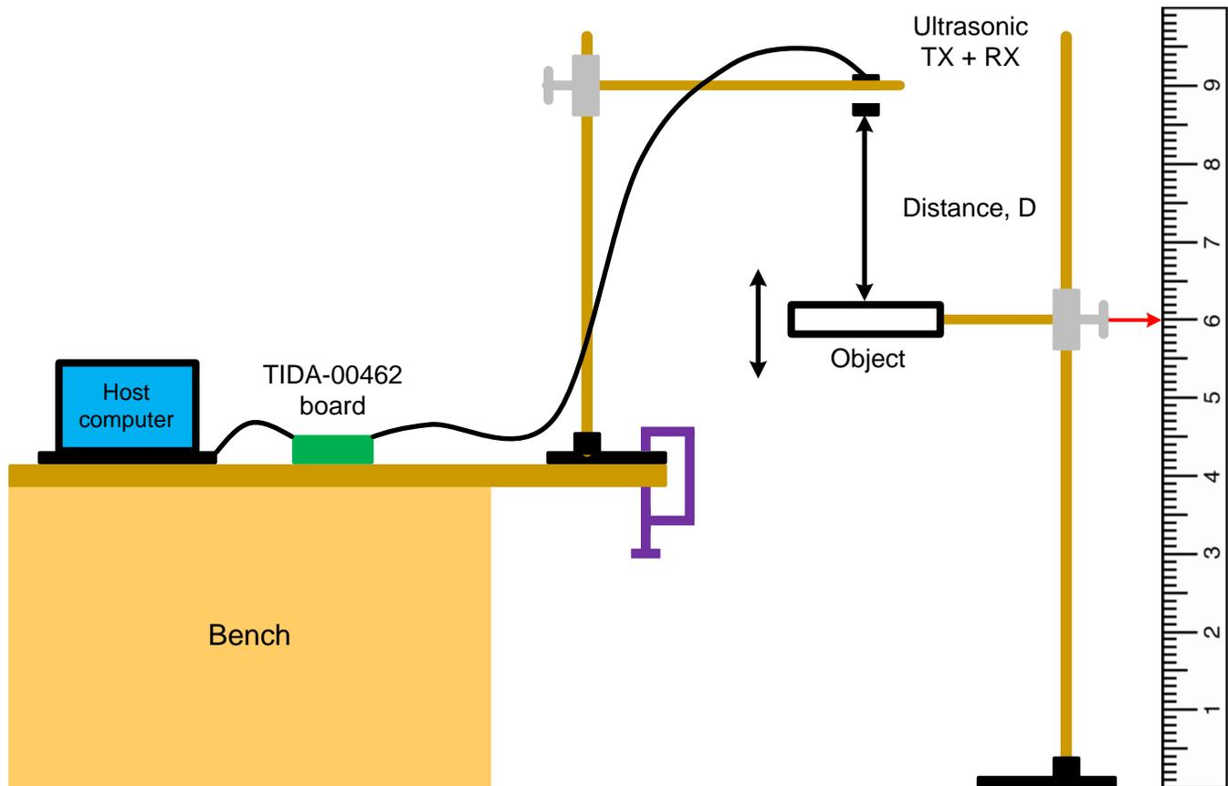
Figure 20. Test Setup
