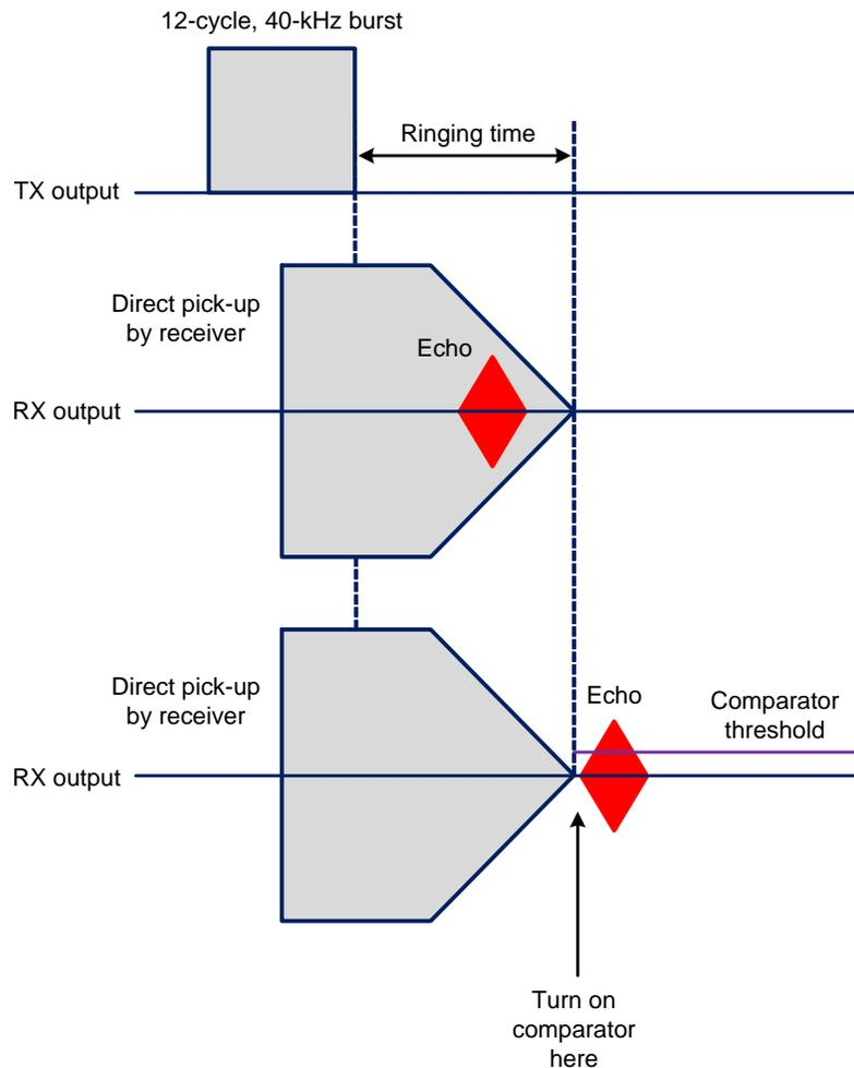
**Figure 14. Ringing and Direct Ultrasonic Wave Pickup**
