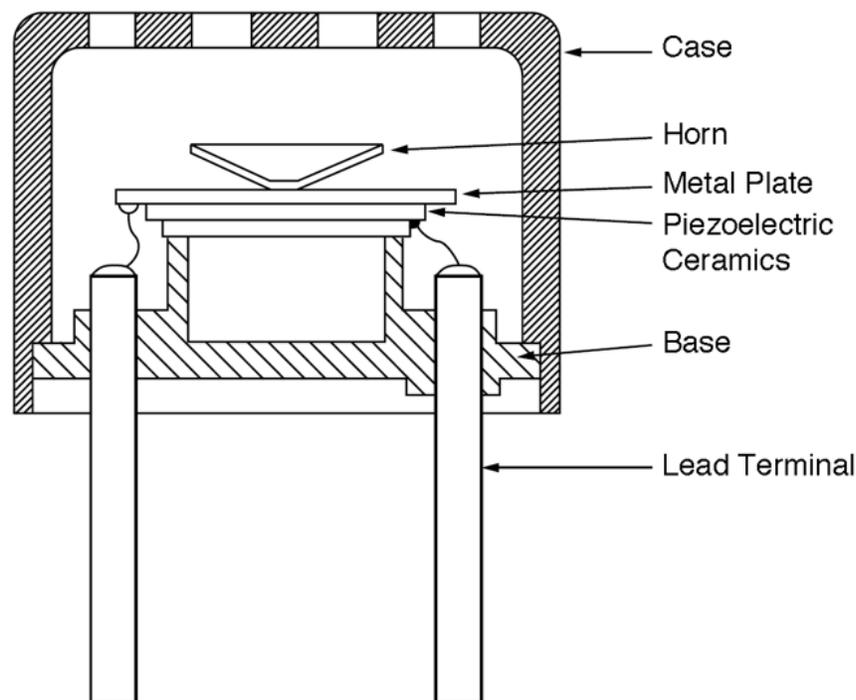
**Figure 8. Ultrasonic Transducer Construction**
