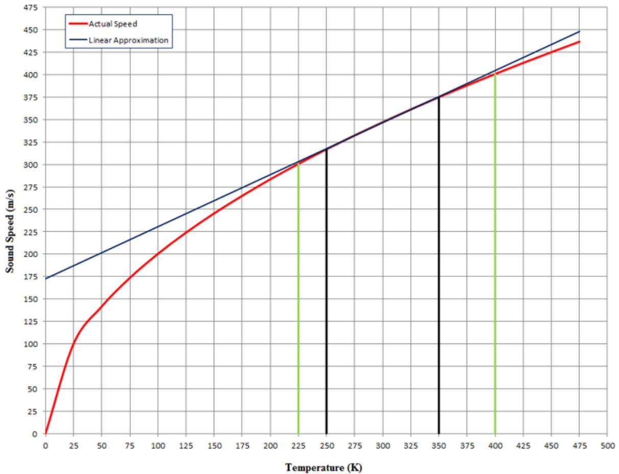
**Figure 6. Speed of Sound versus Temperature**
