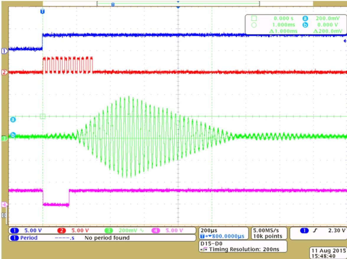
**Figure 16. Oscilloscope Trace of Transmitter's 40-kHz Burst and Direct Wave Pickup**
