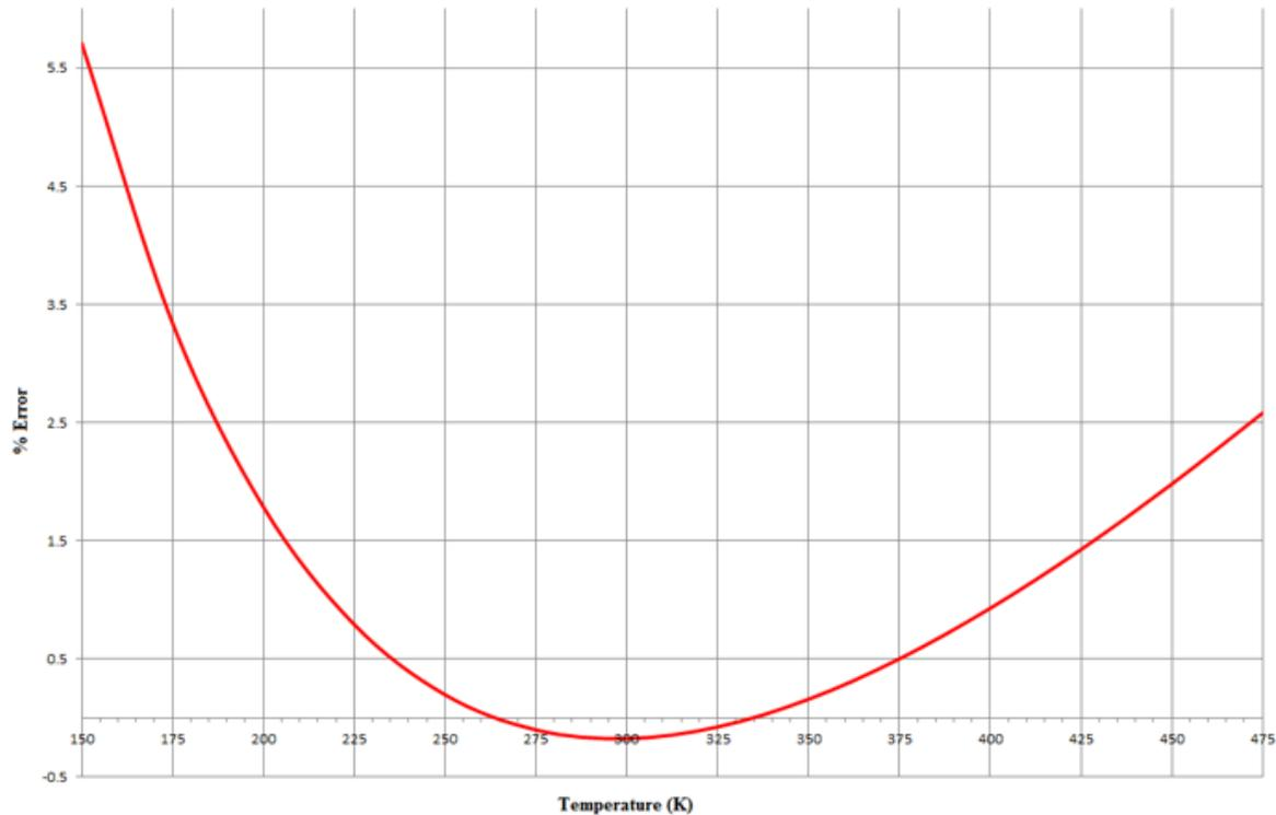
**Figure 7. Percentage Error After Linear Approximation**
