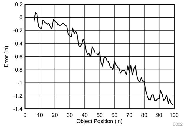
Figure 22. Measured Position Error versus Set Position
