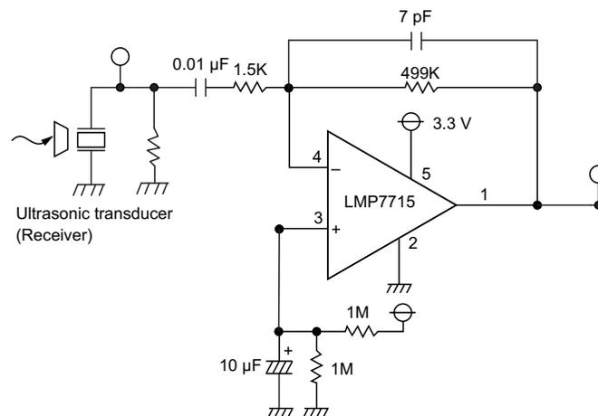
Figure 11. Ultrasonic Receiver Circuitry
