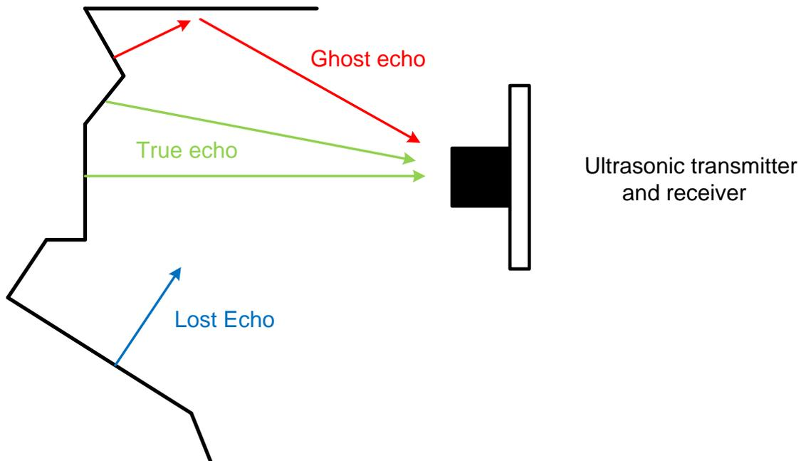
**Figure 5. Echoes From Surfaces at Different Orientations**
