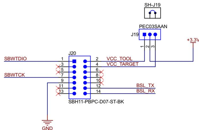
**Figure 19. Spy-Bi-Wire Programming Connections**
