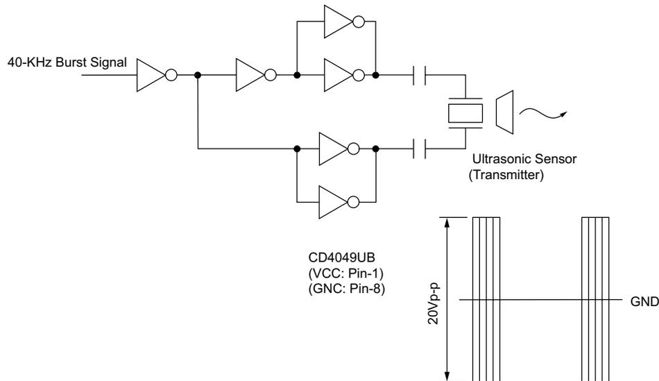
**Figure 10. Ultrasonic Transmitter Circuitry**
