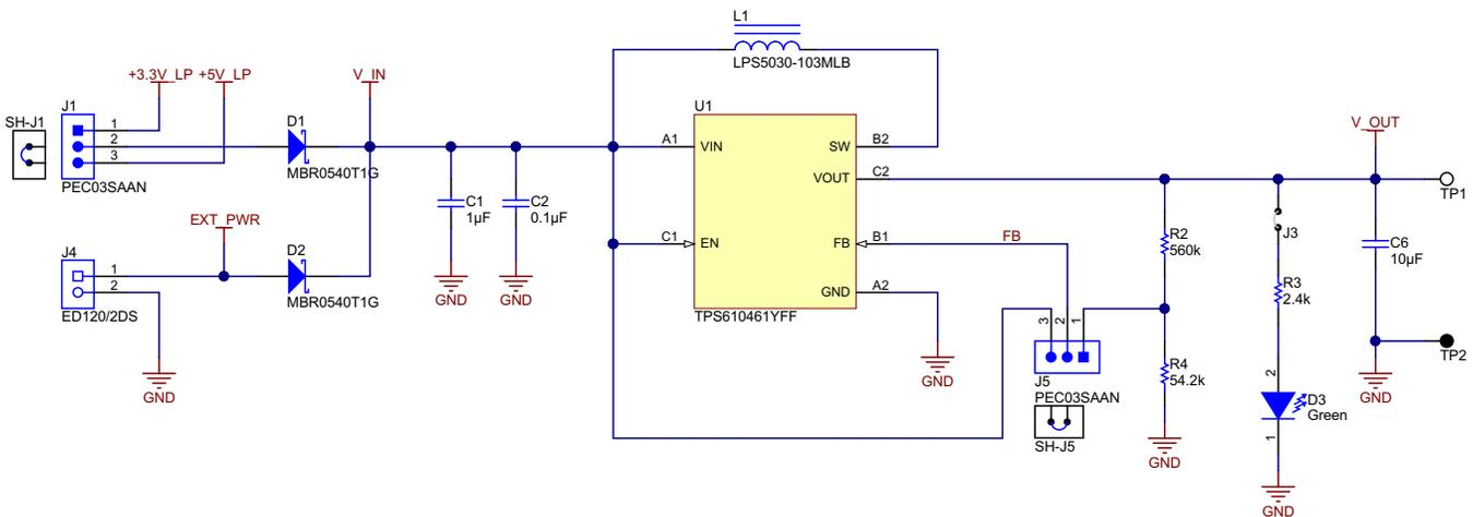
**Figure 12. TPS61046 Boost Converter**
