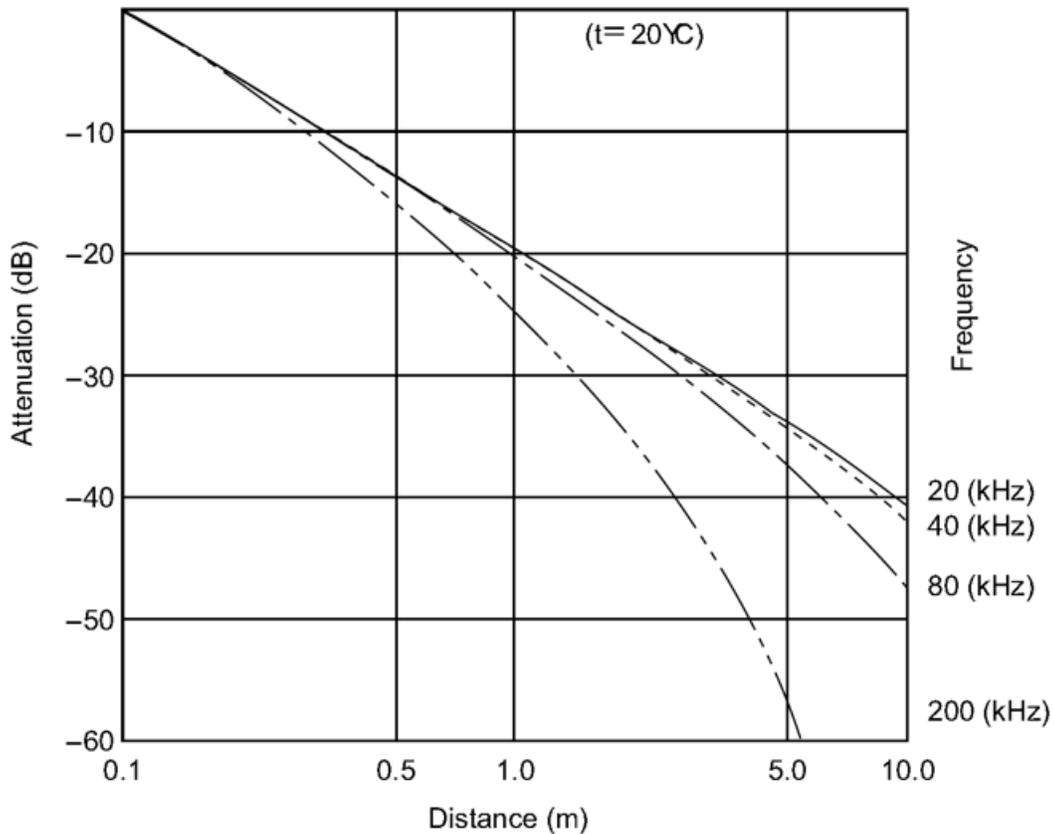
**Figure 4. Attenuation of Ultrasonic Waves With Distance**
